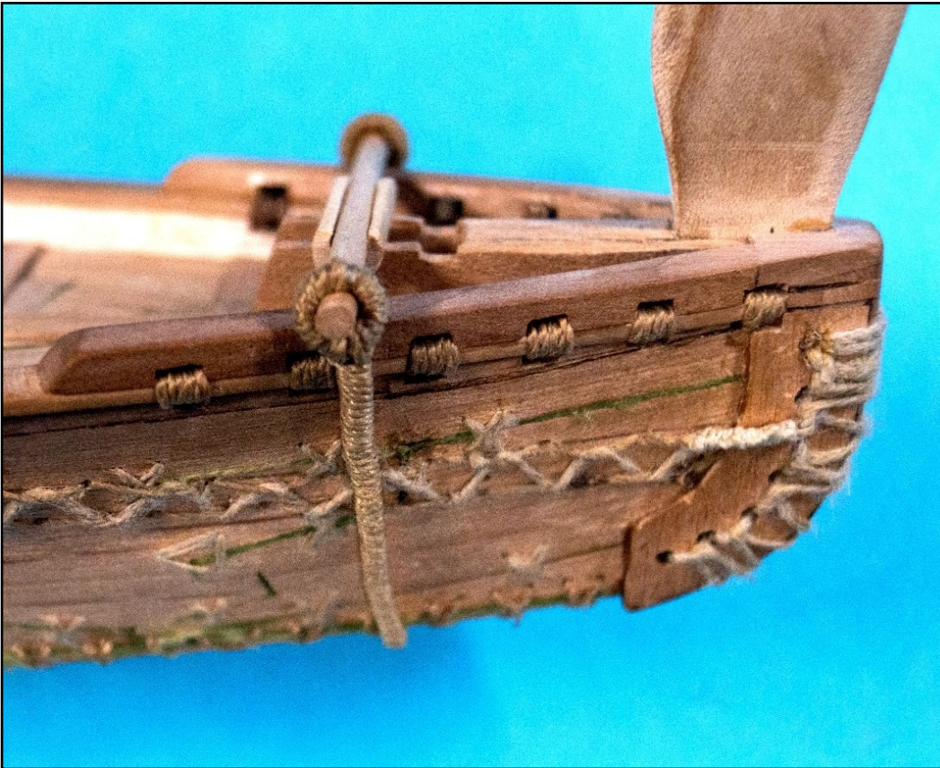
Forward stay completed and test fitted to the bow.
